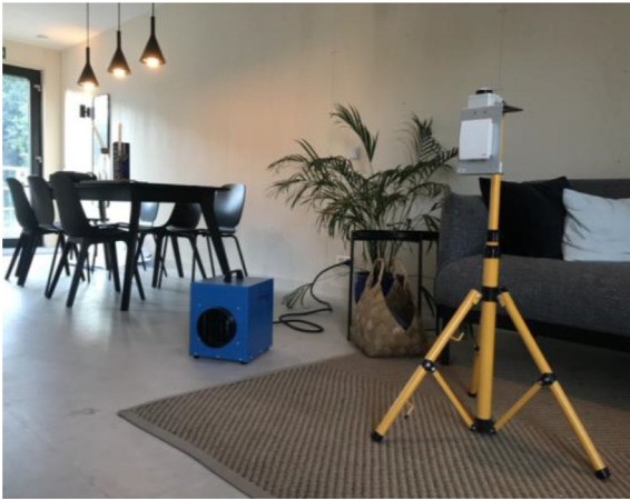
Fig. 9. Example of a room with a fan heater (blue) and a tripod (yellow) with indoor climate measurement equipment in the TU Delft building (TUD).
