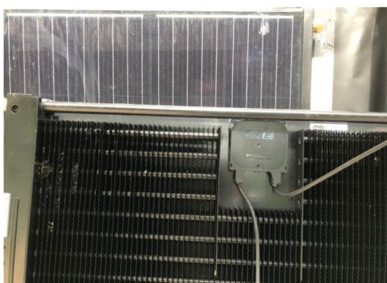
Fig. 24. 375 W PVT collector with additional ambient air heat exchanger on the back (HBC).
